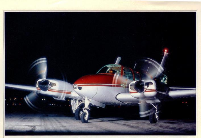
Colemill's performance claims appear to be valid. Initial full-power climb rate at the 99-knot blueline speed was 2,000 fpm. Cruise-climbing at 120 to 130 knots, we were able to maintain a minimum of 1,000 fpm on up to 10,500 feet. Fuel flow in the climb declined from an initial 22 gallons per hour to about
