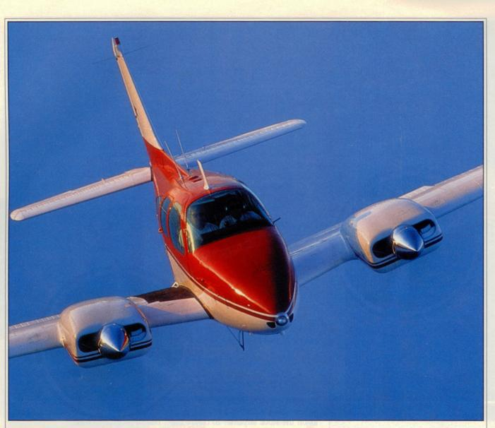
factured 1,700-hour-TBO IO-550-E engines, the President II conversion includes new fuel and oil lines, vacuum pumps, 60-amp alternators, and lord mounts; Hartzell three-blade, 74-inchdiameter props, governors, and spinners; a Shadin digital-display fuel flow computer; and new tachometer with 2,700-rpm redlines. The conversion is priced at \$72,500 with new engines and \$62,500 with remans. The 550s cost about \$12,000 more than the cost of overhauling a pair of IO-470s, according to Colemill.
